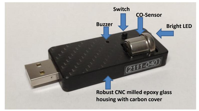
Switch: in Operation: Switch sensitivity >0ppm , 20pp, 50ppm and "LEDs off" in case of no alarm, may be @ night VFR connected @PC: start printout of Memory (Failiure and 3h rolling )
